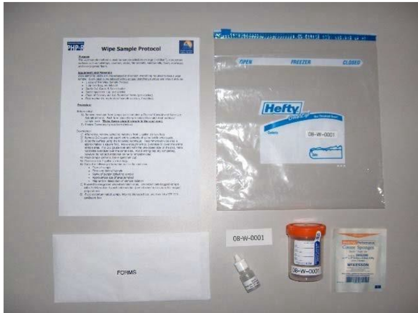
Pictures show one wipe sample kit complete with: Sampling Protocol, State Lab and Chain of Custody Forms, sterile specimen cup, saline bottle, sterile 2x2, secondary (Ziploc bag), and field location marker.
